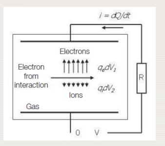
The mode of operation depends on applied voltage (V)
