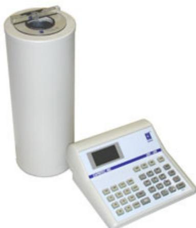
FIG. 9.1. A typical dose calibrator (e.g. CRC 25R).
