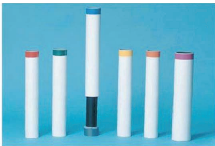
FIG. 10.8. Set of lead-lined plastic sleeves (Calicheck™ Dose Calibrator Linearity Test Kit, Calicheck, Cleveland, OH, USA) for evaluation of dose calibrator linearity by the shield method. The set is supplied with a 0.64 cm thick lead base, a colour coded unlined sleeve (to provide an activity measurement equivalent to the zero time point measurement of the decay method) and a six colour coded lead-lined sleeve providing attenuation factors nominally equivalent to decay over 6, 12, 20, 30, 40 and 50 h, respectively. (Courtesy of Calicheck, Cleveland, OH, USA.)
