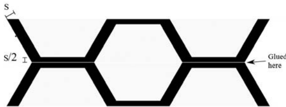
FIG. 11.5. Illustration of fabrication of foil collimator by gluing two stamped lead foils. It should be noted that the foils must be stamped so that the portions of the septa that are glued are half the thickness of the rest of the septa. Furthermore, careful alignment is essential to preserve the hole shapes.
