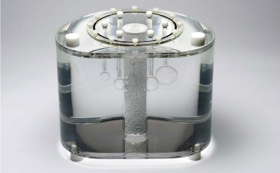
FIG. 15.18. National Electrical Manufacturers Association/International Electrotechnical Commission image quality phantom.
